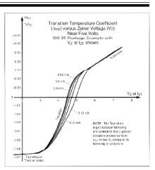
Figure 2. Transition Temperature Coefficient vs Zener Voltage Near Five Volts
